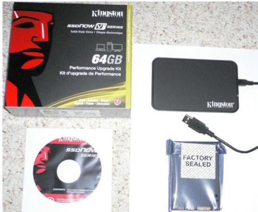
I purchased a Kingston SSDNow V+ Series 64-GB SATA, 3GB/s, 2.5-inch SSD with the notebook upgrade kit from Amazon for about \$160. The kit comes with a 2.5-inch, 64-GB SSD, a USB external hard disk drive (HDD) enclosure and cable, and a CD-ROM that includes the Acronis disk cloning software. The kit also comes with a 3.5-inch mounting kit for desktop computers which I didn't need.
